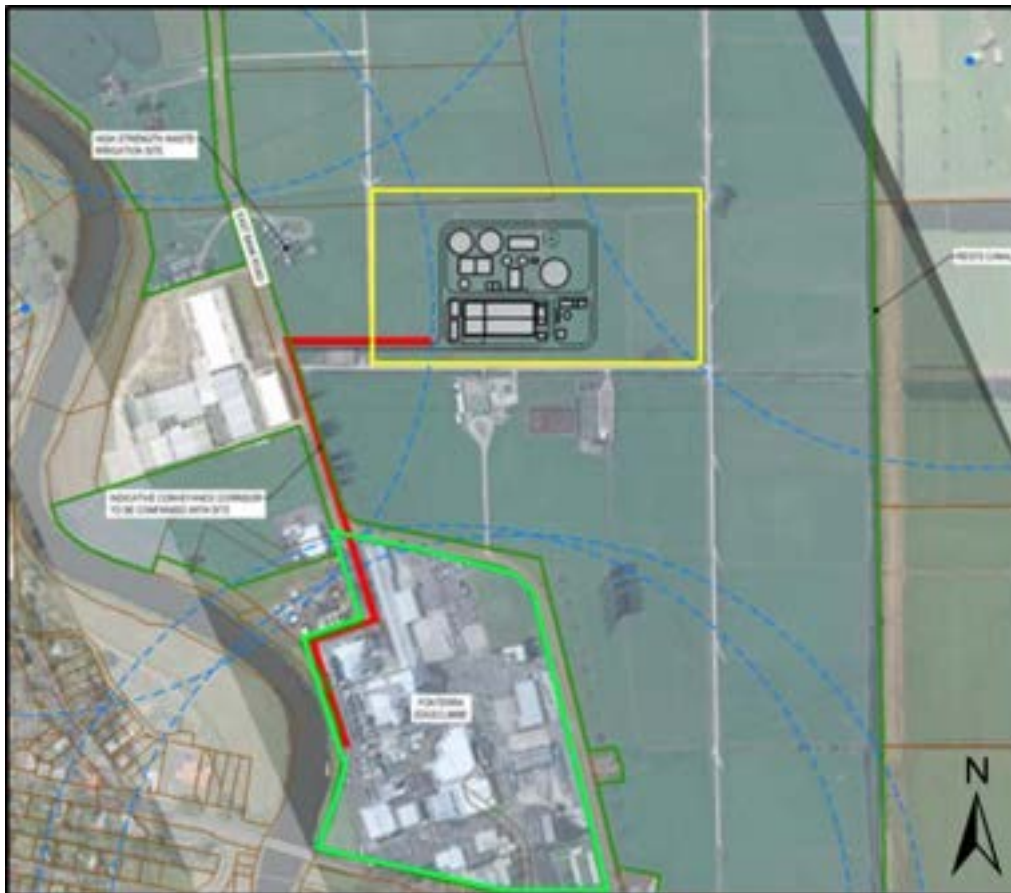
Figure 1b – WWTP overlain on aerial imagery, with associated pipework also assessed as part of this PSI in red. Main boundary of Fonterra Edgecumbe Facility in green. Source: Beca Engineering Project Team ('pre-concept'), May 2022.
